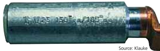
Picture 5: The markings on the cable lug provide information relating to the crimps, the manufacturer, cross section and allocation of cable.
