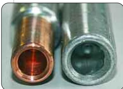
Picture 8: Normally the aluminium section (right) has a larger diameter than the copper section (left) to equalize the poor conductivity of aluminium.
