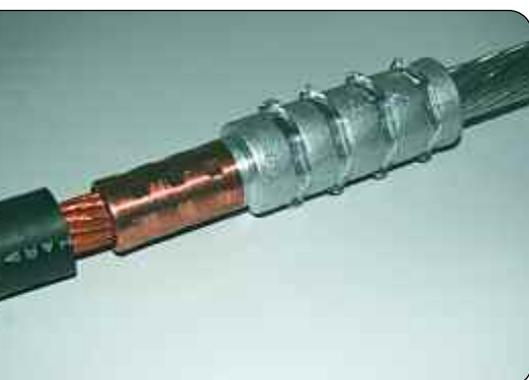
Picture 1: Use of an incorrect crimping die and/or an incorrect crimp will result in an over compression (right) or an under compression (left) and in the worst case in fire.
