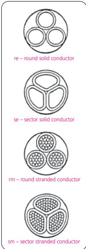
Picture 4: Various shapes of aluminium conductors
